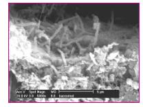
Biofilm layer on EMM® media magnified 5,000X using electron microscope.
