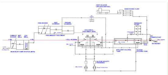
Shown here is an STP using the EMMAS system to maintain receiving river water at Class II of the NWQS as in Table 2 above.
