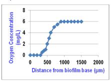
Oxygen profile in biofilm layers, giving anaerobic, anoxic and aerobic conditions in one system, enabling breakdown of a large range of trace pollutants from nutrients to detergents to colouring matters.
